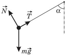
$$\frac{mv^2}{R} = T_1 \sin \alpha - N_1 \cos \alpha, \quad T_1 \cos \alpha + N_1 \sin \alpha - mg = 0. \quad \text{Отсю-}$$
